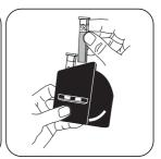
Place sample cuvette in the sample chamber. Positioning on the right side.
