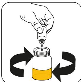
Add drops of **Alkalinity LR Titrant TA3** or **Alkalinity HR Titrant PA2/TA2** to give a **orange/ yellow** colour.
