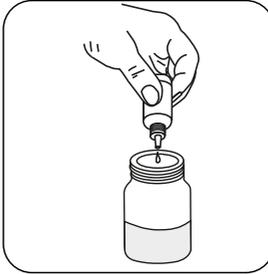
Add **4** drops of **Hardness Calcium Buffer CH2** per **10 mL** of sample.
