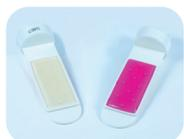
Dipslides for testing in Cooling Water
