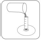
Hold the test tube vertically over a white surface and view downwards on the bottom mark.
