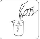
Remove one test strip. Hold Dip the test strip into the solution to be tested so that all pads are completely immersed.
