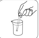
Remove one test strip. Hold Dip the test strip into the solution to be tested so that all pads are completely immersed. (1 second)
