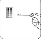
Read the result from the colour scale. (If nitrate ions are present, the outer test paper (at the end of the stick) turns reddish purple. The test field above (towards the end of the handle) shows the nitrite concentration.)
