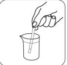
Remove one test strip. Hold Dip the test strip into the solution to be tested so that the pad is completely immersed.
