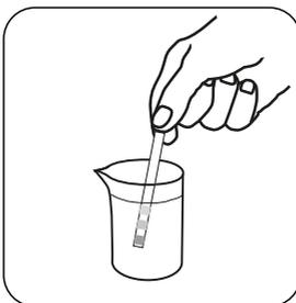
Dip the test strip into the solution to be tested so that all pads are completely immersed.
