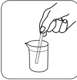
Dip the test strip into the solution to be tested without agitation.
