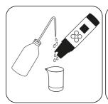
Rinse the electrode with distilled or deionised water and carefully wipe with a paper towel.
