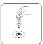
Remove the vial from the sample chamber.
