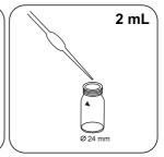
Add exactly 2 mL SPADNS AF reagent solution reagent.
