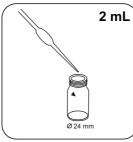
Add exactly 2 mL Note SPADNS AF reagent solution to the 24 mm vial.
