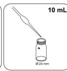
Add exactly 10 mL deionised water to the blank.
