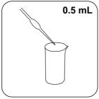
Place **0.5 mL Reagenz Pb-1** in a suitable sample vessel.
