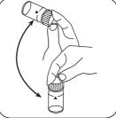
Dissolve tablet(s) by inverting.
