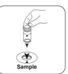
Fill 24 mm vial with 10 mL Close vial(s). sample.
