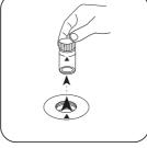
Remove the vial from the sample chamber.
