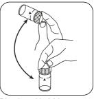
Dissolve tablet(s) by inverting.
