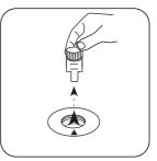
Remove vial from the sample chamber.
