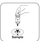
Fill 24 mm vial with 10 mL Close vial(s). sample.
