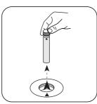
Remove vial from the sample chamber.
