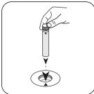
Place the supplied Zero vial Press the **ZERO** button. (red sticker) in the sample chamber. • Pay attention to the positioning.
