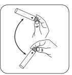
Add 2 mL 1,00 N Sodium Close vial(s). Hydroxide solution to the digested sample.
