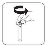
Open a digestion vial PO<sub>4</sub>-P Acid Reagent.
