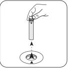
Remove vial from the sample chamber.
