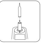
Place the ampoule in the sample chamber.
