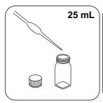
Fill the digestion vial with 25 mL sample.
