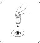
Remove the vial from the sample chamber.
