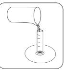
Hold the test tube vertically over a white surface and view downwards on the bottom mark.
