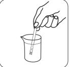
Remove one test strip. Hold Dip the test strip into the solution to be tested so that all pads are completely immersed.
