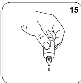
Adicionar **15 gotas KS278 (50% sulfuric acid)**.
