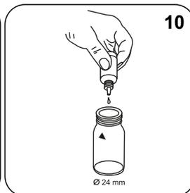
Adicionar **10 gotas Hardness Total Buffer TH2**.
