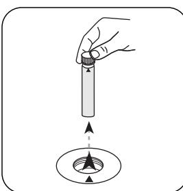
Remove **vial** from the sample chamber.
