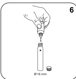
Add **6 drops H<sub>2</sub>O<sub>2</sub>-Reagent Solution**.
