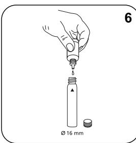
Add **6 drops H<sub>2</sub>O<sub>2</sub>-Reagent Solution**.
