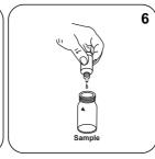
Add 6 drops DPD 1 Buffer Add 2 drops DPD Solution to the sample vial.
