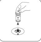
Remove the vial from the sample chamber.
