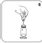
Add 6 drops DPD 1 Buffer Add 2 drops DPD Solution to the sample vial.
