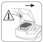
Remove the vial from the thermoreactor. (Note: vial will be hot!)
