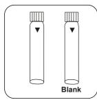
Prepare two reaction vials. Put 0.2 mL deionised Mark one as a blank.
