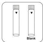
Prepare two reaction vials. Put 2.5 mL deionised Mark one as a blank.
