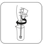
Crush tablet(s) by rotating slightly and dissolve.
