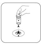
Remove the vial from the sample chamber.
