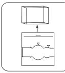
Remove **vial** from the sample chamber.
