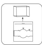
Remove **vial** from the sample chamber.
