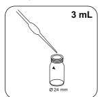
Put 3 mL deionised water Put 3 mL sample in the in the blank.
